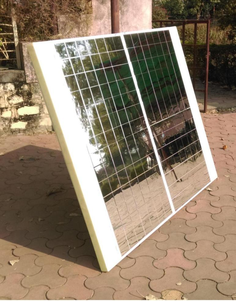
A heliostat (from helios, the Greek word for sun, and stat, as in stationary) is a device that includes a mirror, usually a plane mirror, which turns so as to keep reflecting sunlight toward a predetermined target, compensating for the sun's apparent motions in the sky.
