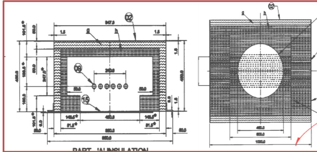
CAVITY LINEAR RECEIVER APPLIED FOR 30kWt PILOT PLANT OF CL-CSP
