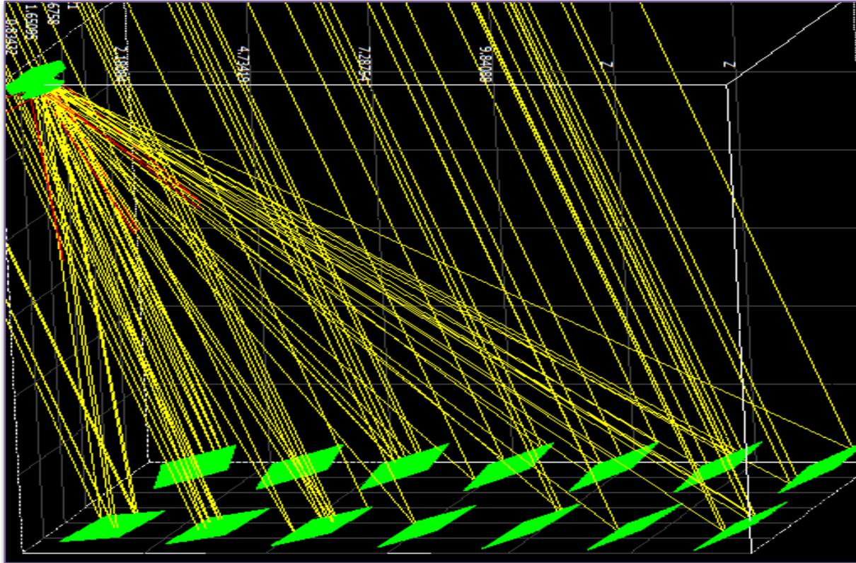
**Ray tracing for 14 heliostats on 3 April 2017 at 12:15PM**
