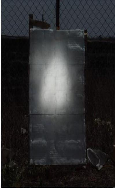
The test was carried out 8:30am using the ceramic board screen placed perpendicular toward sun position. The focal image was taken by the camera at lower sensitivity.
