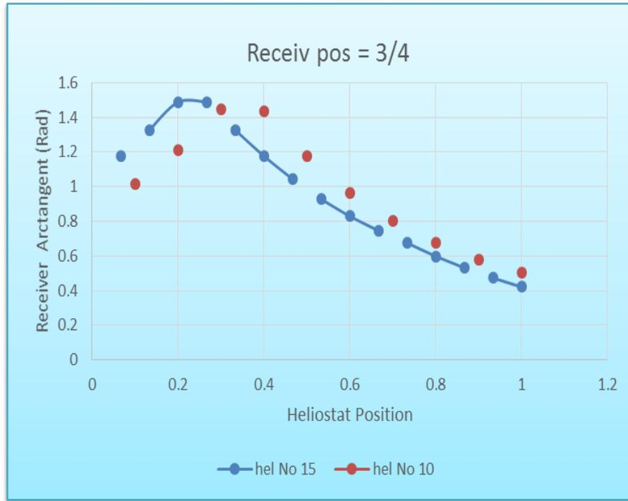
**Relationships of the arc tangent and the normalized heliostat number between the reduced case of Table 2.2-22 (HelNo=3/4) (Curve with red circle; heliostat number=10) and the design point of Table 2.2-32 (HelNo=3/4) (Curve with blue circle; heliostat number=15)**
