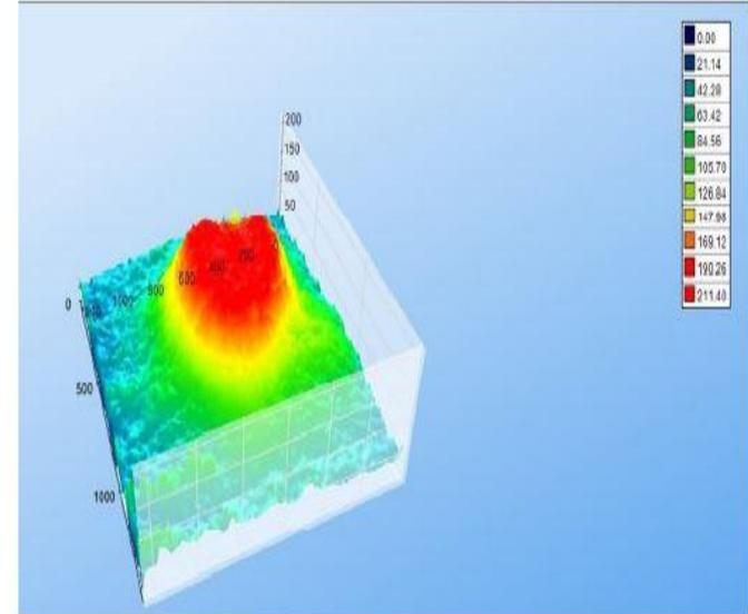
The analysis of the flux intensity showed that the highest flux area diameter is around 55cm which is smaller than 60cm of the 2ndary reflector.
