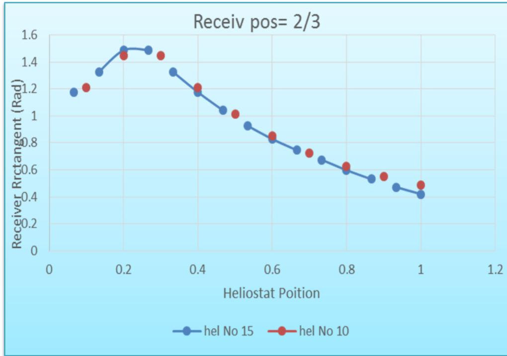
**Relationships of the arc tangent and the normalized heliostat number between the reduced case of Table 2.2-32 (HelNo=2/3) (Curve with red circle; heliostat number=10) and the design point of Table 2.2-32 (HelNo=3/4) (Curve with blue circle; heliostat number=15)**
